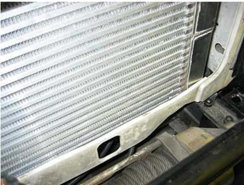
Here you can see the front panel in place with the removed edge. Make sure it is not sharp because it might otherwise damage the intercooler core. The front panel on my vehicle is a bit bent and butchered but if you've got a straight one it will look better (see picture above).
