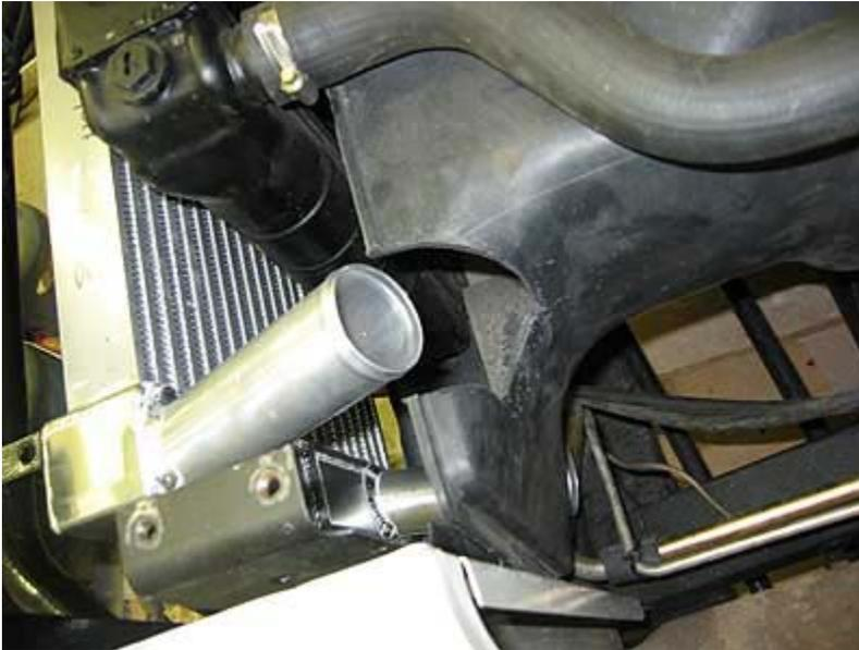
For both pipes (top and bottom) I did have to cut out the plastic.
