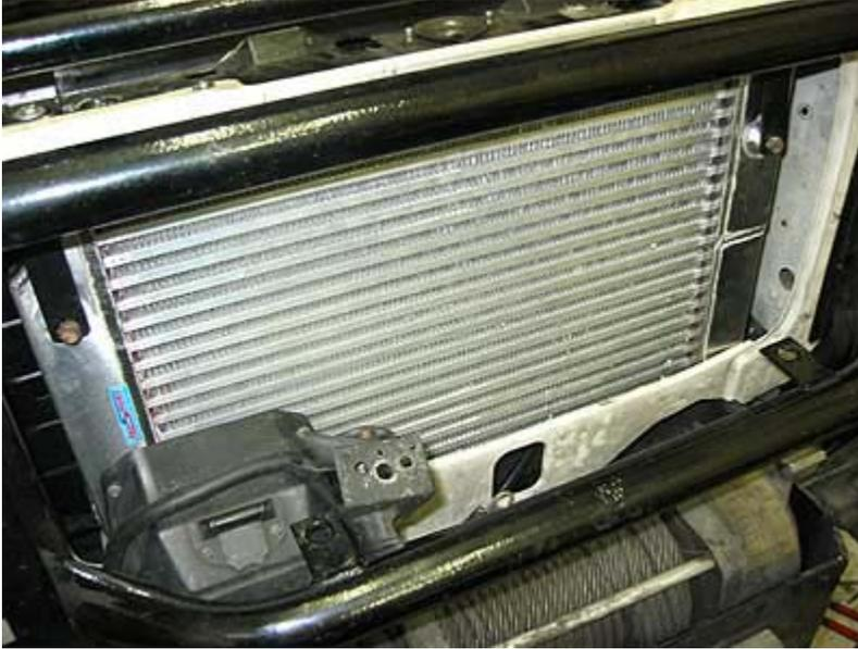
It is difficult to see because of the bull bar but the two top supports are at the left and right corner (see picture above). Making these fit properly did cost me most time of the job.
