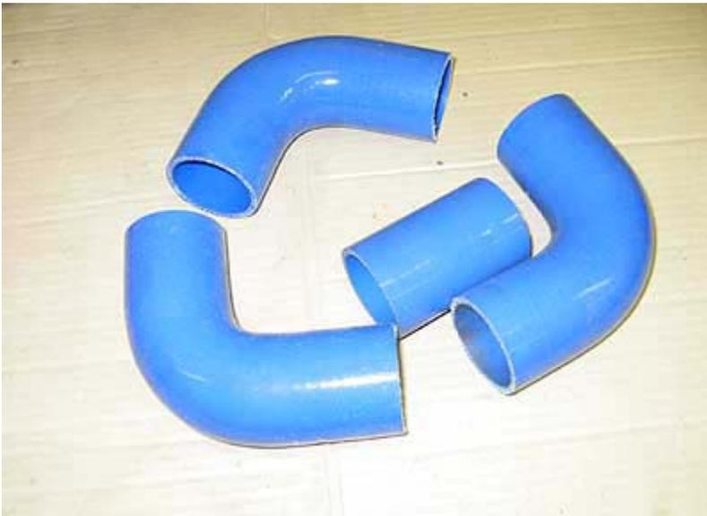
I should have received two straight ones and two bend ones but the kit above is for the standard 200Tdi intercooler. The 2nd straight hose I did need to fit the full size intercooler was send to me later by Andrew from Allisport FOC.
